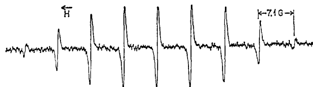
Figure 8. Spectrum probably due to (\text{HOCH}_2)_2\text{NO} during photolysis of a methanol solution at 33^\circ containing 16.6 g of \text{KNO}_2 and 83 ml of \text{H}_2\text{O} per liter.
